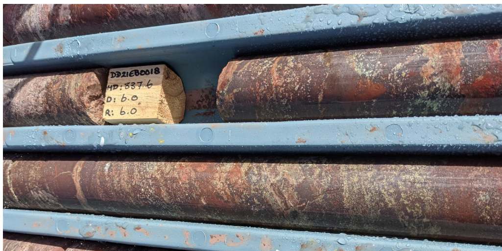
Figure 1 Typical alteration and copper sulphides in the chalcopyrite zone, within the broader 50m zone of primary interest.
