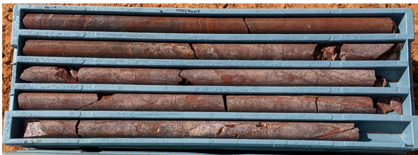
Figure 15 Haematite alteration continues to attenuate, becoming less pervasive and largely restricted to fractures. Silica alteration remains strong. Note that core tray follows directly after Figure 14, and finishes approximately 200m downhole from the unconformity shown in Figure 7.
