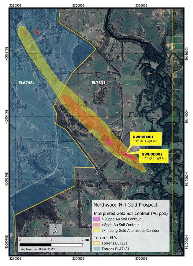
Figure 2 – Location of the first 2 drill holes at Northwood Hill overlying the 5km long gold anomalous corridor and project magnetics
